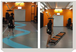
A state-of-the art overground body weight support system allows active movements through a wide range of natural locomotor activities. This system provides optimal bodyweight support while ensuring safety of the participants to prevent falls.
